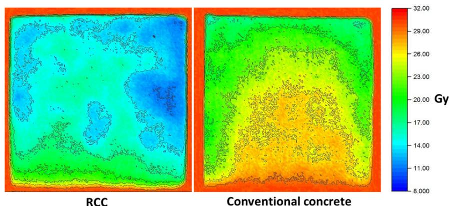
Figure 5 – Qualitative comparison of the shielding of gamma radiation of samples of RCC (left) and conventional concrete (right). The blue color means the lower dose measured at the radiochromic film (higher shielding) and the red color the higher dose (lower shielding).
