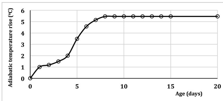
Figure 3 – RCC adiabatic temperature rise (cement with 50% granulated blast furnace slag).
