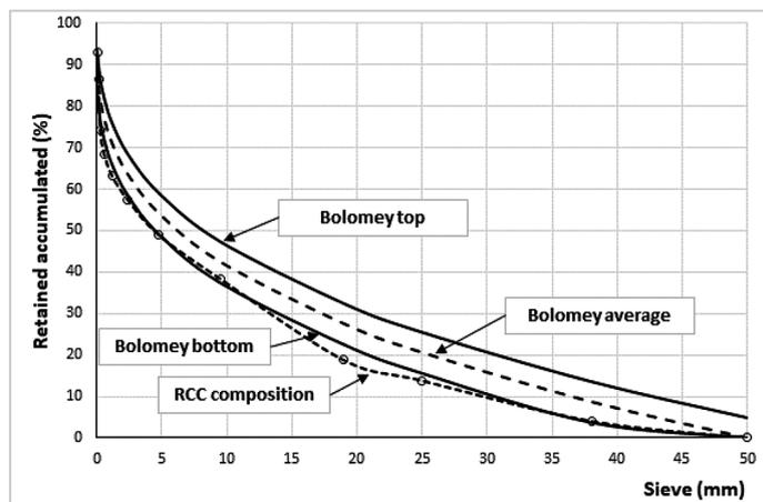
Figure 2 – Granulometry of the RCC aggregate composition compared with the Bolomey curves.
