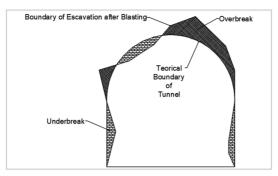
Figure 1 - Real and theoretical section of a tunnel.
