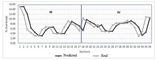
Figure 4 - Values of predicted and real % overbreak along the sections of the tunnel.
