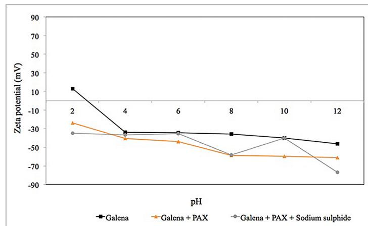
Figure 4 - Zeta potentials of galena treated with PAX ( $10^{-4}$  mol/L) and a mixture of 50 % of the PAX solution plus 50 % of sodium sulphide solution ( $10^{-4}$  and  $10^{-2}$  mol/L) as a function of pH.
