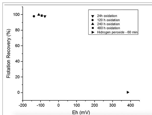
Figure 2 - Floted (%) of oxidized surface galena, at pH 9.5, in different ambience exposure periods (time) and with extremely anodic potential promoted by hydrogen peroxide, in the presence of PAX ( $10^{-4}$  mol/L), in function of the system Eh.
