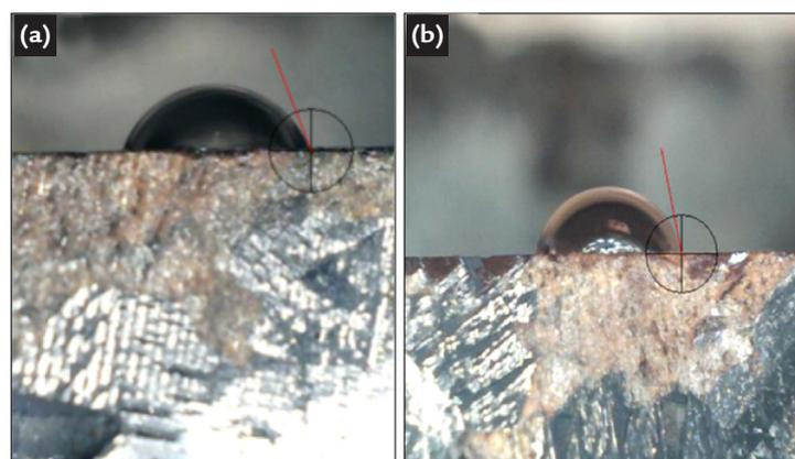
Figure 7 - Images of the measurements of the contact angles on galena for the amyl xanthate solution ( $10^{-4}$  mol/L) treatment. (a) natural galena surface  $\theta = 69^\circ$ ; (b) oxidized galena surface  $\theta = 84^\circ$ . Magnified 4 x.
