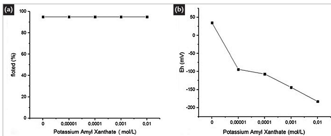
Figure 1 - (a) Floted (%) non-oxidized surface galena recovery, at pH 9.5, in the absence of the collector and under different PAX concentrations, and (b) Eh of the system, in the absence of the collector and under different PAX concentrations, under the same conditions.
