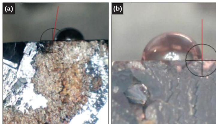
Figure 6 - Images of the measurements of the contact angle on galena for distilled water. (a) natural galena surface  $\theta = 81^\circ$ ; (b) oxidized galena surface  $\theta = 90^\circ$ . Magnified 4 x.
