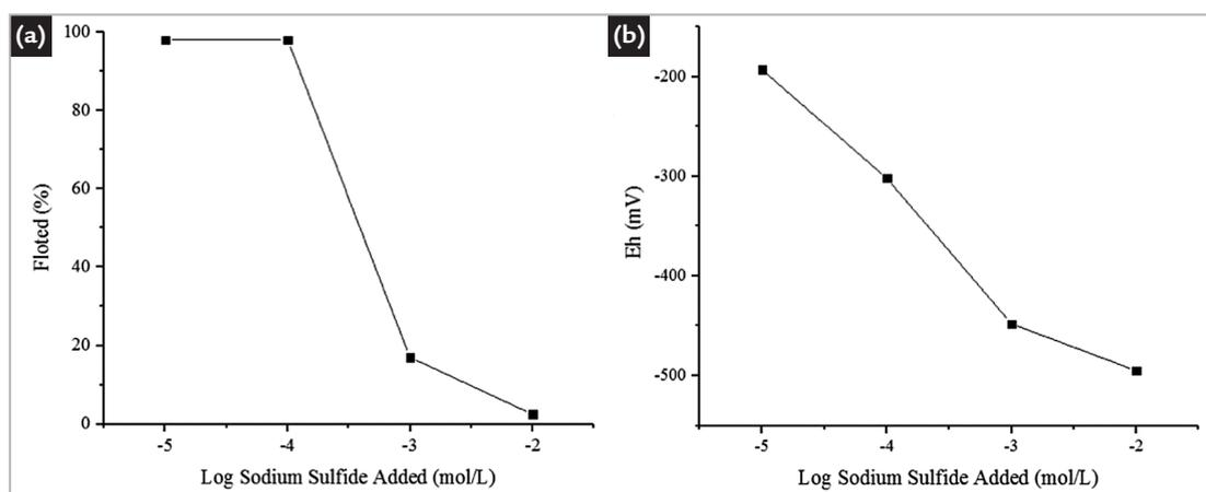
Figure 3 - (a) Floted (%) of non-oxidized surface galena at pH 9.5, in the presence of the collector potassium amyl xanthate ( $10^{-4}$  mol/L), in function of different concentrations of added sodium sulphide and (b) system Eh in function of different concentrations of added sodium sulphide – under the same conditions.
