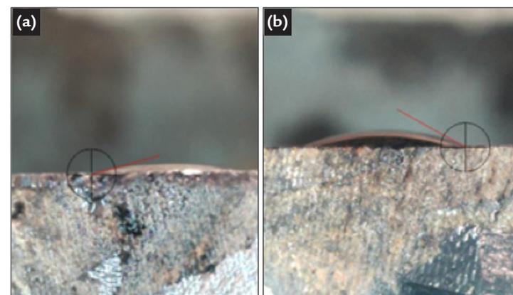
Figure 8 - Images of the measurement of the contact angles on galena for the amyl xanthate ( $10^{-4}$  mol/L) + sodium sulphide ( $10^{-2}$  mol/L) treatment. (a) surface of natural galena  $\theta = 13^\circ$ ; (b) oxidized galena surface  $\theta = 22^\circ$ . Magnification 4 x.
