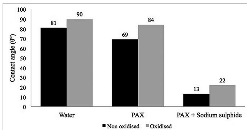
Figure 5 - Contact angles of the oxidized and non-oxidized galena surfaces, measured in the presence of distilled water, amyl xanthate solution, and amyl xanthate + sodium sulphide solution, at pH 9.5.
