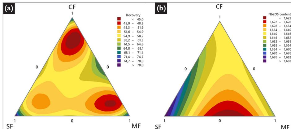
Figure 1 - Contour plot of the flours dosage for niobium (a) recovery and (b) content.
