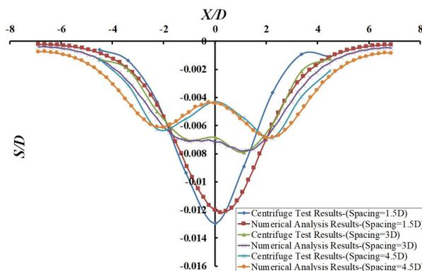
**Figure 3.** Verification of the numerical analysis results through the centrifuge test results of center-to-center spacing of 1.5D, 3D and 4.5D ( $X/D$ : Horizontal distance from center of twin-tunnel (or center of strongbox)/Diameter of the tunnel,  $S/D$ : Vertical settlement of the ground surface/Diameter of the tunnel).
