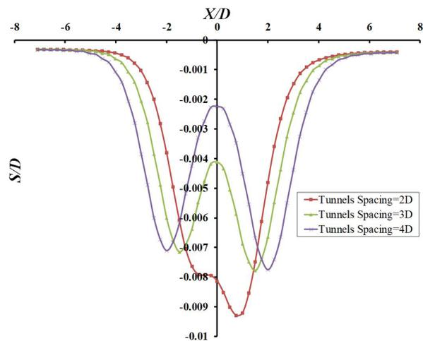
Figure 8. Numerical results of the asymmetric ground surface settlement curves generated by asynchronous excavation of the twin-tunnel (H=10 m and D=6 m).
