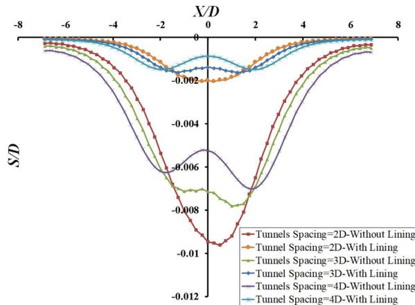
**Figure 11.** Numerical results of the amount and the shape of the surface settlements in the presence of tunnel lining comparing with the asymmetric excavation condition of twin-tunnel (for  $H=10$  m and  $D=4$  m).
