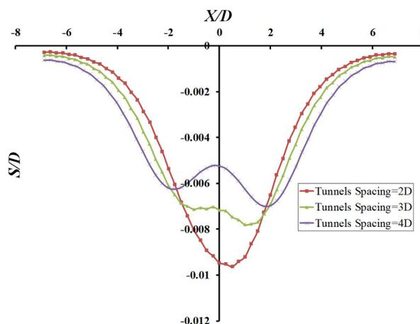
**Figure 7.** Numerical results of the asymmetric ground surface settlement curves generated by asynchronous excavation of the twin-tunnel ( $H=10 \text{ m}$  and  $D=4 \text{ m}$ ).
