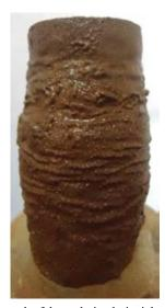
**Figure 16.** Photograph of the undrained triaxial test result of a loose specimen (~78%) of flotation tailings (BL-2&1).
