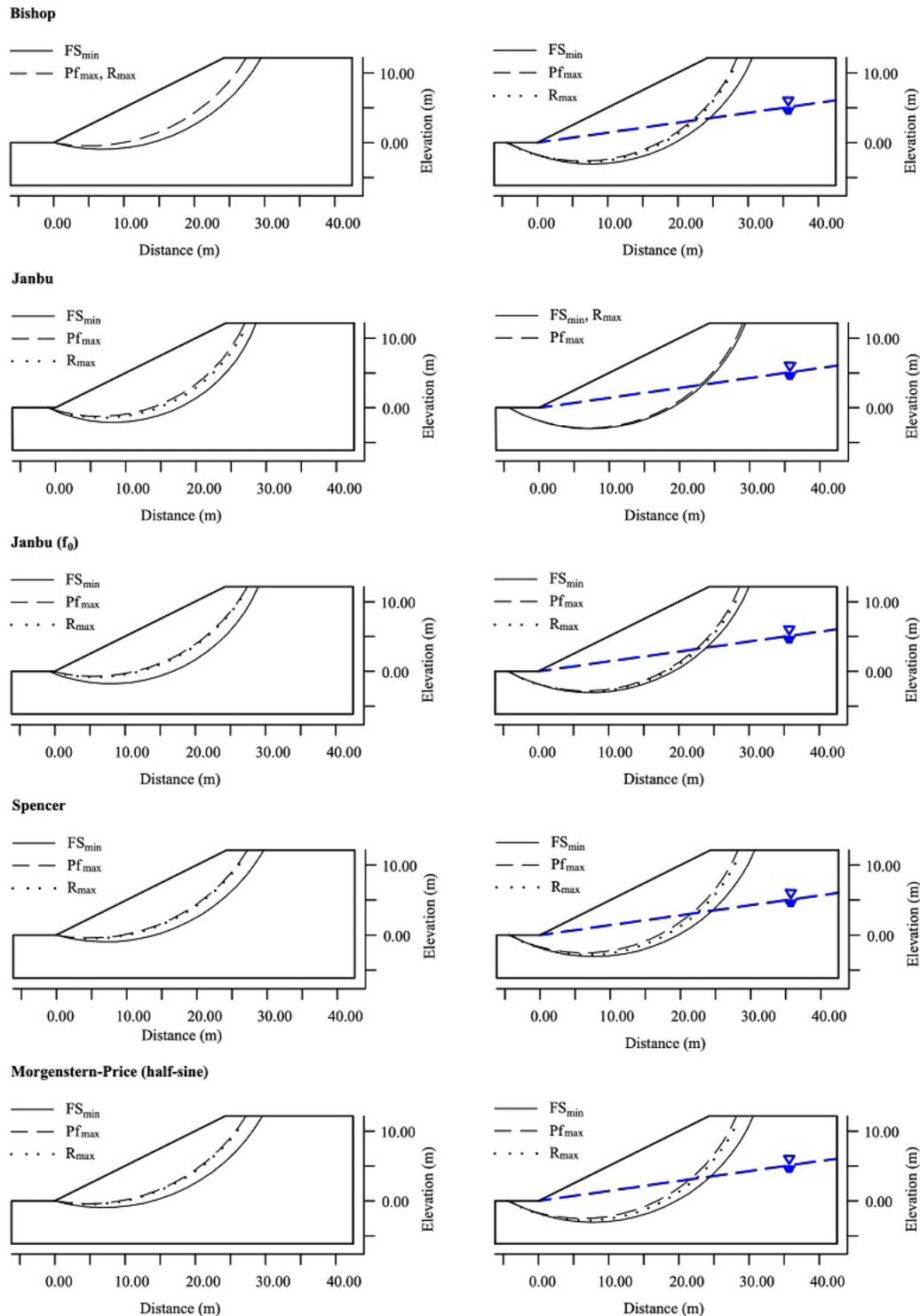
Figure 2. Deterministic and probabilistic critical slip surfaces.
