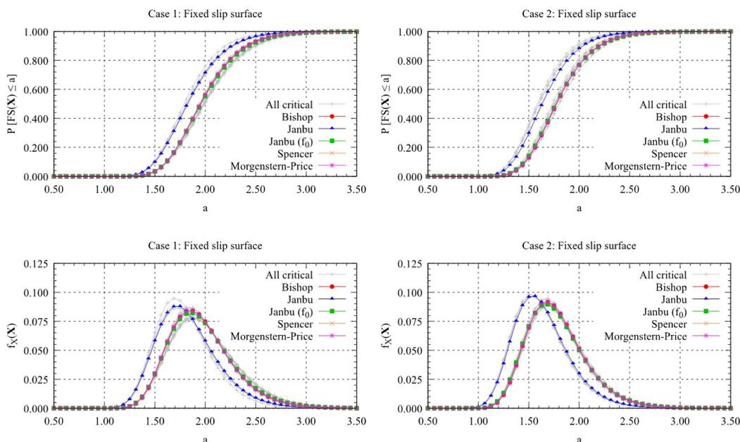
**Figure 6.**  $FS(X)$  probability distribution curves of the fixed slip surface and all critical surfaces.
