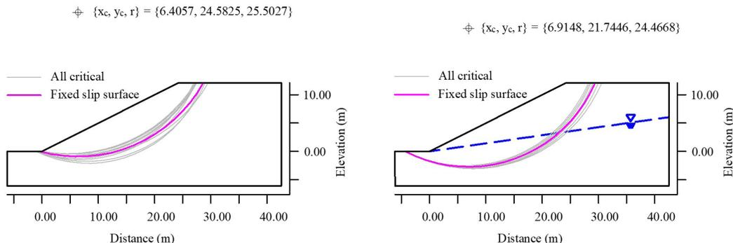
**Figure 5.** An overlap of all critical surfaces identified by deterministic and probabilistic criteria and different limit equilibrium methods employed in direct coupling.
