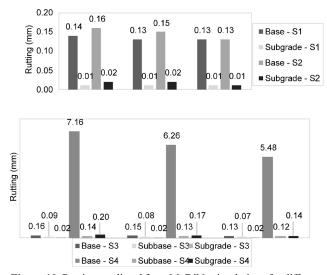
**Figure 10.** Rutting predicted from MeDiNa simulations for different traffic levels and pavement structures using the Acre laterite gravel in the composition of the base or subbase layers.
