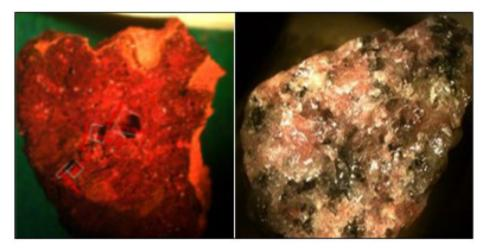
**Figure 5.** A microscopic image (magnification factor of 6.5) of (a) a sample of the Acre laterite gravel evaluated in this study and (b) a sample of crushed granite for comparison.
