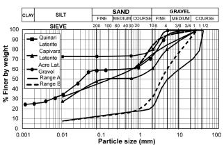
**Figure 2.** Gradation distributions of three Acre laterite gravels, including the one evaluated in this study, and two gradation envelopes from the Brazilian standard DNIT 098 (DNIT, 2007).
