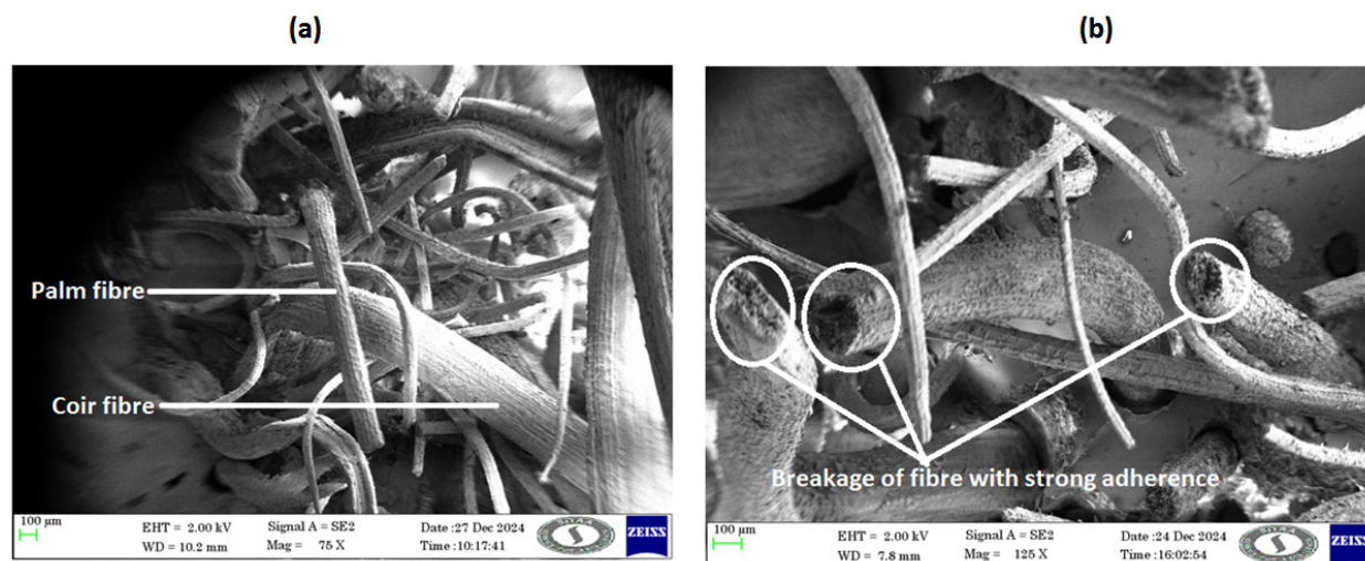
Figure 3. SEM image of VIE composites loaded with 30% Borassus flabellifer and Cocos nucifera fibre during tensile fracture.
