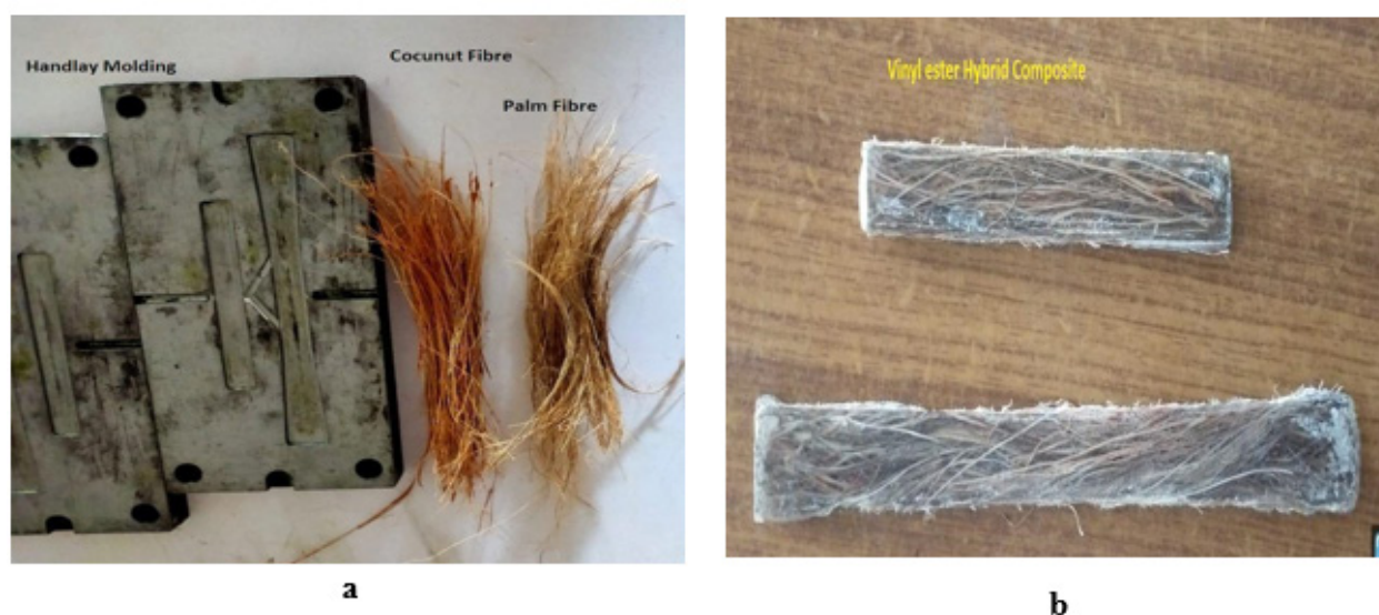
Figure 1. a) Representation of utilized handlay molding, extracted Borassus flabellifer and Cocos nucifera fiber b) Representation of developed VIE composites.
