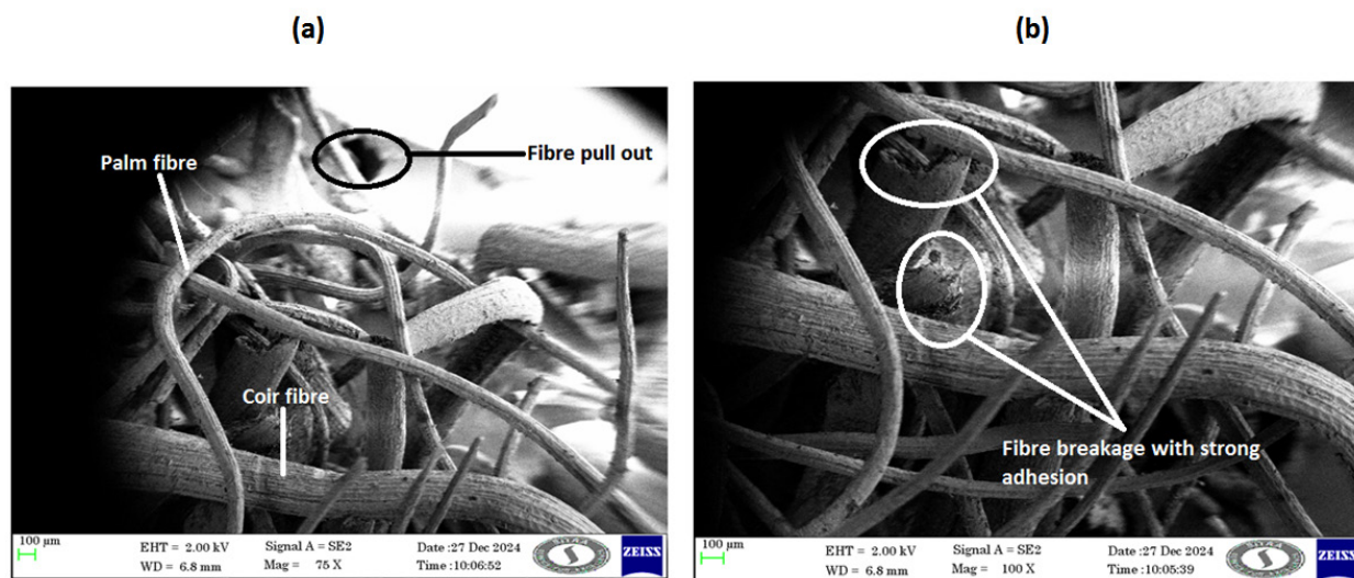
Figure 4. SEM image of VIE composites loaded with 30% Borassus flabellifer and Cocos nucifera fiber during flexural fracture.
