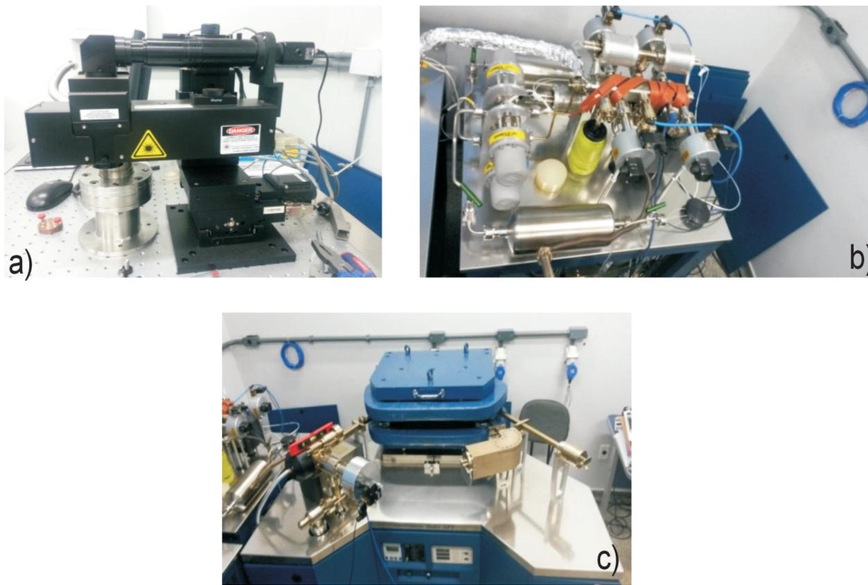
**Figure 1** - Photograph of the gas extraction, purification and measurement system; (a) laser heating system, (b) gas purification bench, and (c) Helix-SFT noble gas mass spectrometer.
