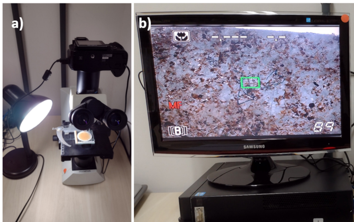
Figure 1. Optical microscope used for the initial location of microplastic fragments: a) filter positioned in the microscope and, b) image obtained by optical microscope with an increase of 100 x.
