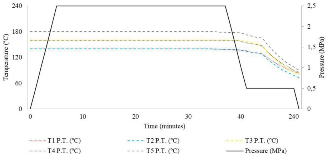
**Figure 1.** Diagram of the thermomechanical densification process with the temperatures of the hydraulic press (P.T. = Press temperature).
