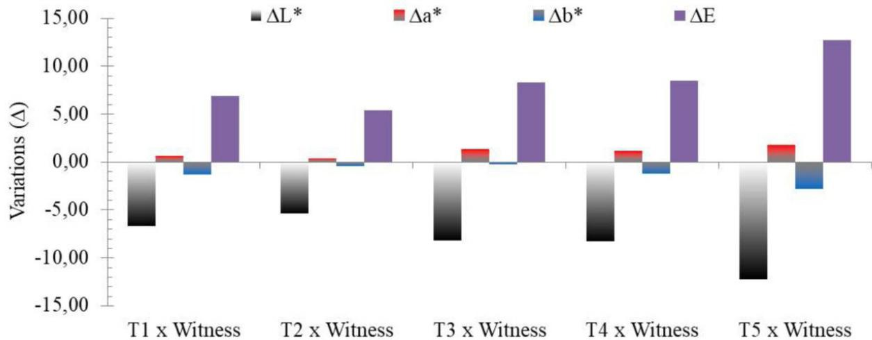
**Figure 4.** Variations between the values of the colorimetric parameters of the wood samples of *Gmelina arborea* after the application of the treatments in relation to the control wood.
