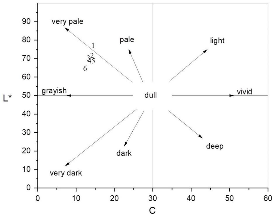
**Figure 3. Diagram of luminosity ( $L^*$ ) x saturation ( $C$ ) of *Gmelina arborea* samples in natural condition and treated. Note: 1=Control; 2=T1; 3=T2; 4=T3; 5=T4; 6=T5.**
