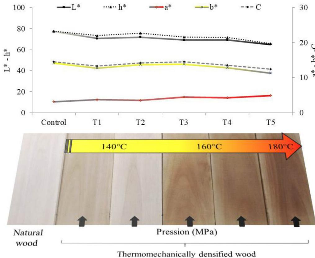
color of wood has become less vivid and with greyish appearance, as the temperature of the treatments increases. The above changes can be observed in the  $L^* \times C$  diagram (Figure 3).
