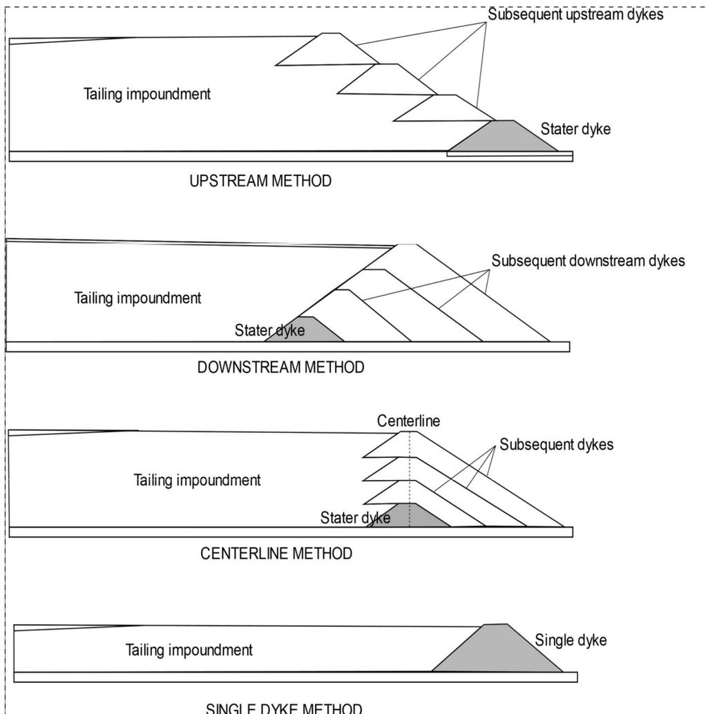
**Figure 1.** Construction methods of tailing dams.
