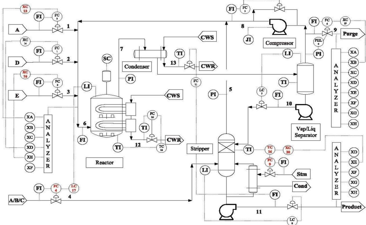
Figure 7. Piping diagram of the Tennessee Eastman process.
