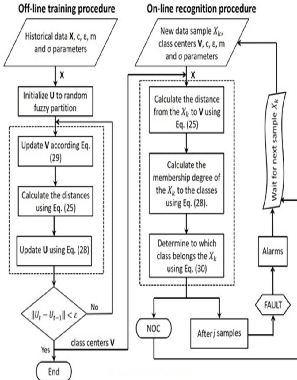
**Figure 5.** Flowchart of the condition monitoring process.
