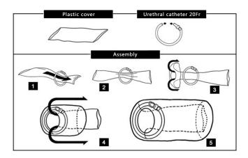
FIGURE 1 – Materials and assembly of the protective device
