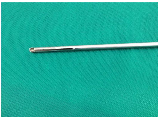
Figure 4. Toggle applicator tip. Leaked tube with cut-out at the tip for wire fitting, 0.5mm wall thickness, 50cm long and 5mm diameter. Inside is another stainless steel cylinder with 3.5mm to push the "toggle".
