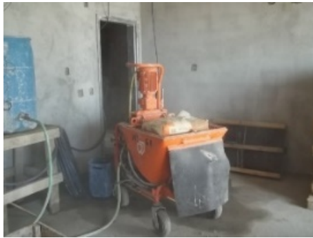
Figure 3 - Sprayer Equipment PFT G4 - construction work B
