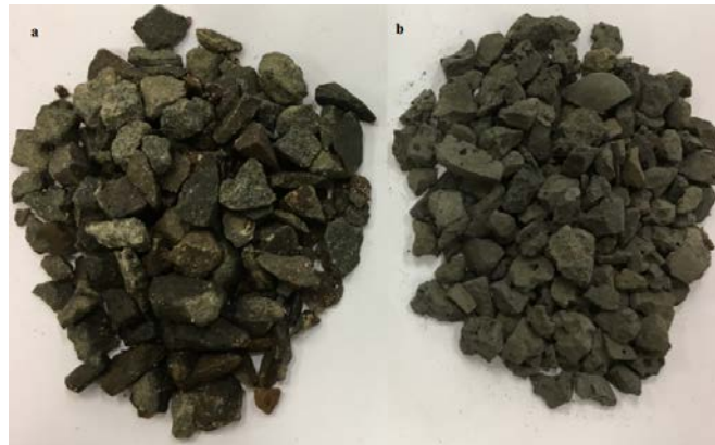
Figure 3 - (a) Natural aggregate and (b) EAF aggregate appearance
