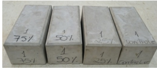
Figure 6 - Paving blocks with 75%, 50%, 25% and 0% of EAF aggregate incorporation after curing for 56 days
