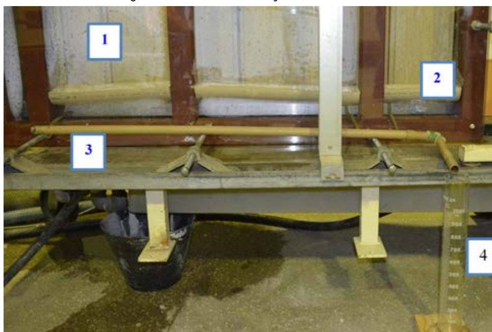
Figure 11 - Device for collecting water in the drainability test
