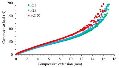
The elongational stress profile ( $\sigma_B$ ) and elongational viscosity ( $\eta_B$ ) over shear rate ( $\dot{\epsilon_B}$ ), according to equations 2 to 4 (STEFFE, 1996), was based on the results of compressive load vs compressive extension and presented in Figure 9.
