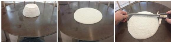
Figure 3 - Flow table test
