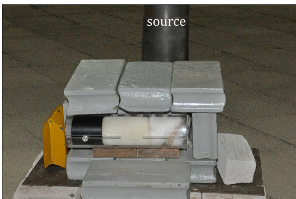
Figure 3 - Protection plumb device that did not cover the back of the animal.
