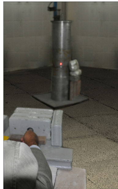
Figure 4 - Laser used to determine the beam axis.
