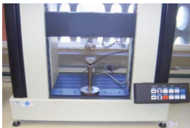
FIGURE 1 - Computerized mechanical test machine used in the tensile strength tests
