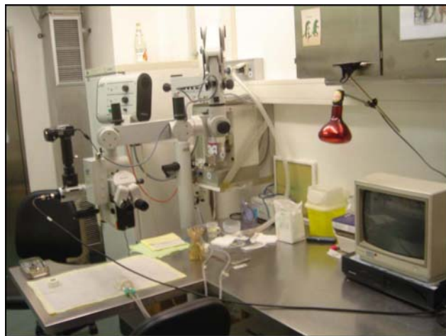
FIGURE 1 - Example of a microsurgery training unit with a surgical microscope connected to a digital camera and video-monitor system
