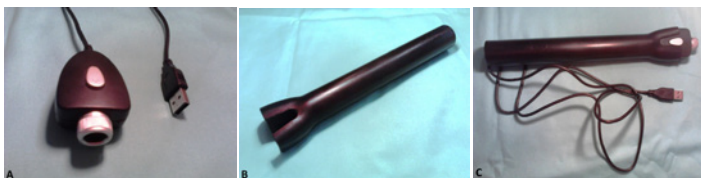
FIGURE 5 – Preparation of webcam. A. Original Webcam. B. Support for handling. C. Webcam with support for handling coupled and cable to connection.
