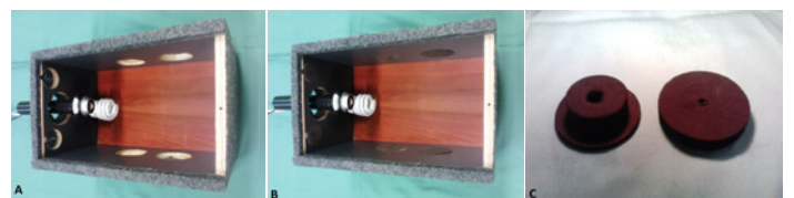
FIGURE 3 – Box and closures. A. Box without covers in the holes. B. Box with covers in the holes. C. Rubber closures for the holes.
