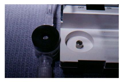
**FIGURE 7** - Membrane sensitive to pressure that transmits the measurement of pressure to the manometer device.
