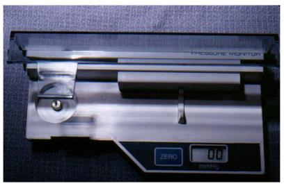
FIGURE 6 - Electronic manometer device.
