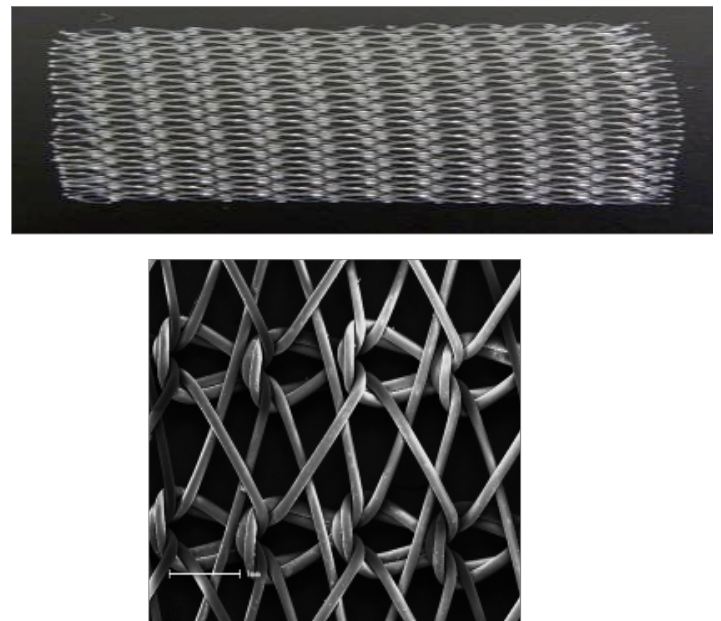
FIGURE 1 – Polypropylene mesh on normal and electron microscopy scanning aspects.
