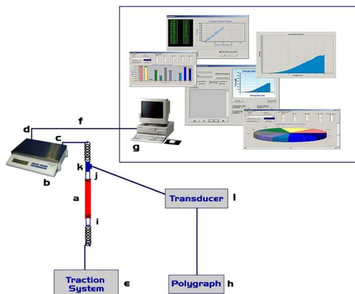
**FIGURE 1** - Schematic representation of ETR. **a)** descendent colon segment, **b)** precision balance, **c)** strength cell, **d)** serial port, **e)** traction system, **f)** serial communication cable and SABI 2.0, **g)** computer with serial interface and SABI 2.0, **h)** polygraph, **i)** catheter cannon (closed light), **j)** catheter cannon (open light), **k)** triple-via plug attached to the supporter and **l)** polygraph transducer
