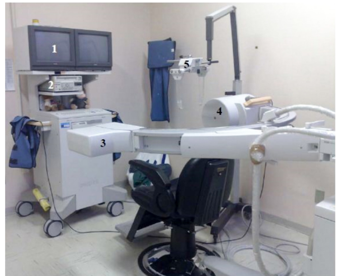
Figure 3. Videofluoroscopy system: TV monitors (1), video-recording system (2), X ray unit (3) ray image intensifier (4) and cephalostat (5)
