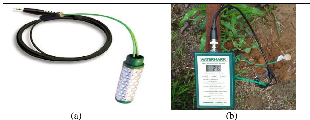
Figure 2. (a) Watermark TM soil tension sensor and (b) Watermark TM equipment for reading soil water potential ( \Psi_m ).
