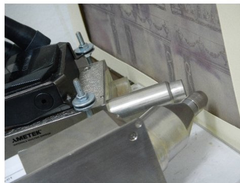
Figure 5 - Images of measurements being made with portable XRF systems used in the analyses at USP - IFUSP Institute of Physics (left, Ag tube) and the IPEN Energy and Nuclear Research Institute (right, Au tube). Item Pharmacy Labels , IHF Collection. Photo: the authors.
