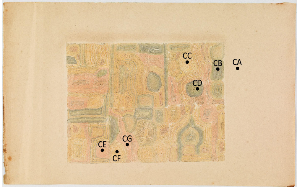
Figure 14 - Distribution map of points CA to CG, measured on item Inimitable paper of the IHF Collection, analyzed with IFUSP's ED-XRF portable system (Ag tube).
