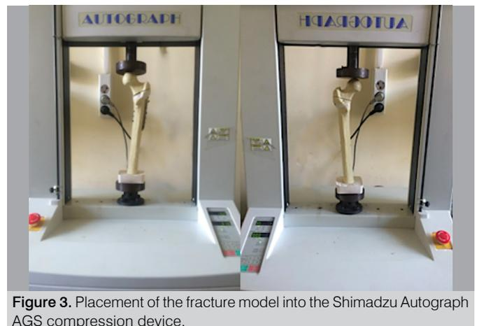
**Figure 3.** Placement of the fracture model into the Shimadzu Autograph AGS compression device.
