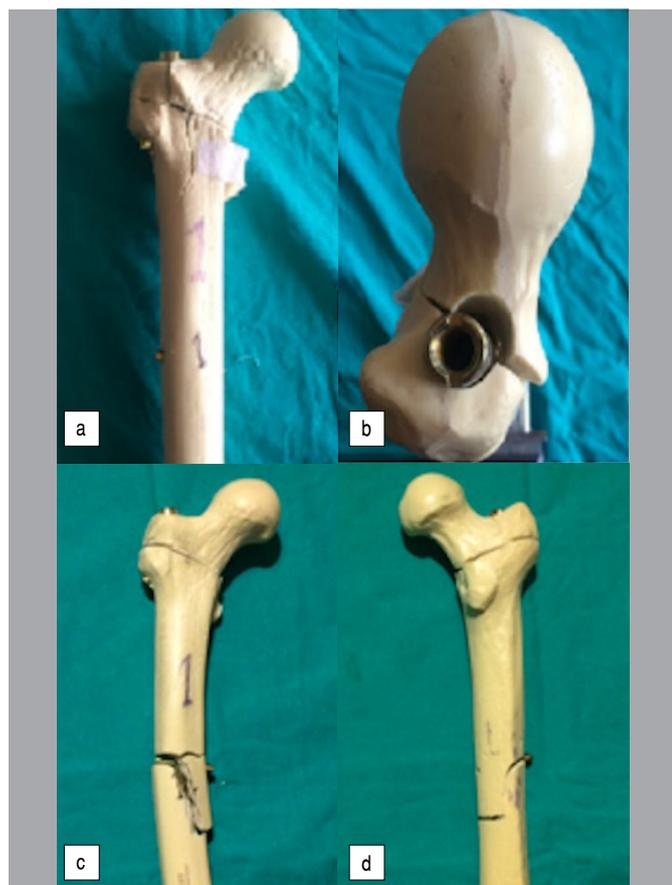
**Figure 4.** Fracture patterns in the antirotator proximal femoral nail group after testing. A: new fracture line from the entry point, anterior view; B: new fracture line from the entry point, axial view; C: butterfly fragment and new oblique fracture line, anterior view; D: butterfly fragment and new oblique fracture line, lateral view.
