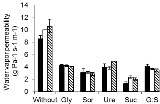
Figure 2 - Water vapor permeability ( \text{g m}^{-1} \text{ s}^{-1} \text{ Pa}^{-1} ) of oat starch films at different thickness. ■ 80 \mu\text{m} ; □ 100 \mu\text{m} ; ▨ 120 \mu\text{m} . Without = without plasticizer; Gly = glycerol; Sor = sorbitol; Ure = urea; Suc = sucrose; G:S = glycerol:sorbitol.
