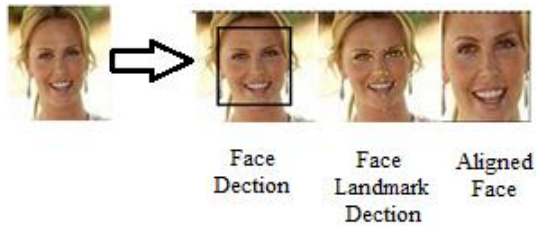
Figure 2: Pre-processing steps for face image retrieval system
