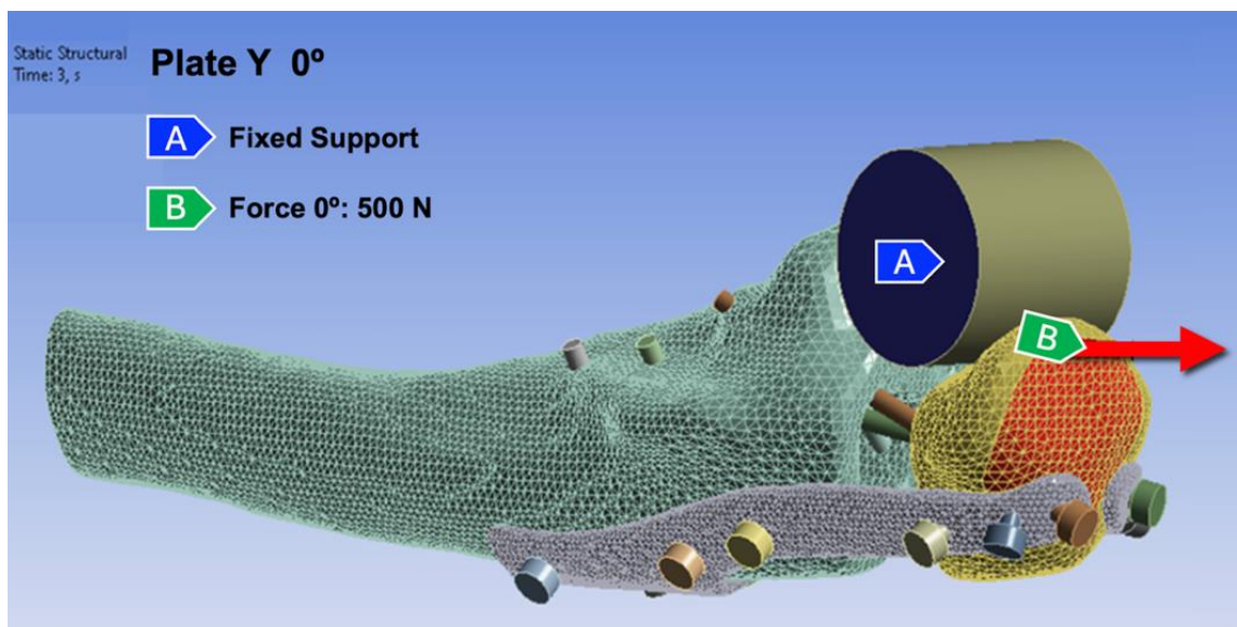
Figure 4. Image showing the application and direction of Force (B, red arrow) on the Y plate system at 0° elbow flexion, in Ansys® software. Source: the authors
