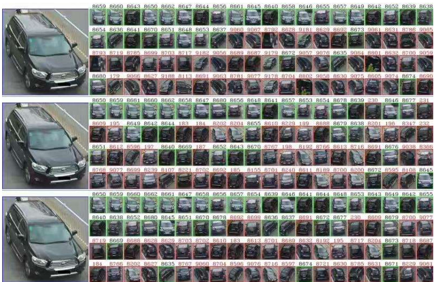
Figure 2. Comparison of re-identification results between different features with different dimensions. The vehicle image with the same vehicle ID and camera ID as the query image is removed. The top, middle and bottom are the re-identification results of features with dimensions of 512, 2048 and the fusion of these two features, respectively. They are ranked according to the Euclidean distance from small to large, and each ranking result only displays the top 80 matching images. On the left is the same query image, and on the right is the query results. The green boxes are the positive images of the query image, and the red boxes are the negative images of the query image. The number above given in each small image is the original number of the vehicle image in the gallery set.
