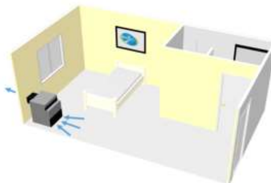
Figure 2. Best simple suggestion, using portable HEPA equipment - Compact decontamination unit.
