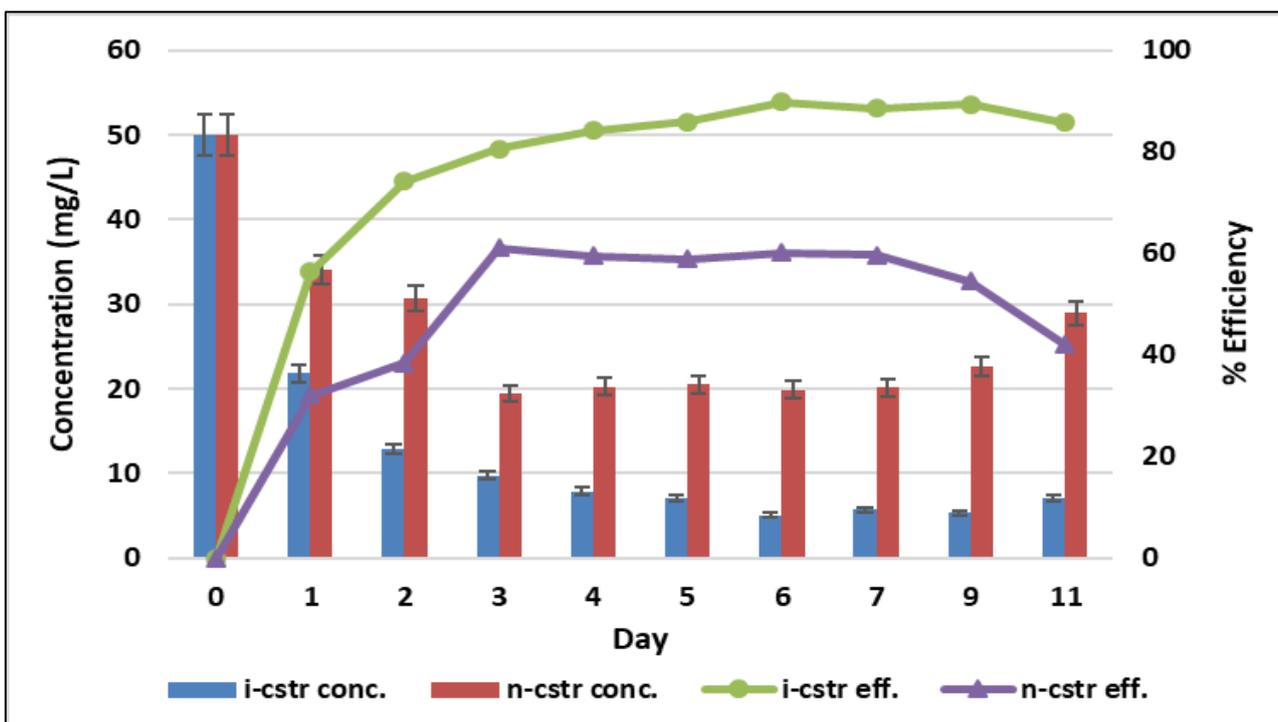
**Figure 4.** The graph shows the concentrations of TA determined in the effluent during the degradation and the removal efficiencies. (i-cstr: inoculated CSTR with degradative isolates, n-cstr: non-inoculated CSTR as control).
