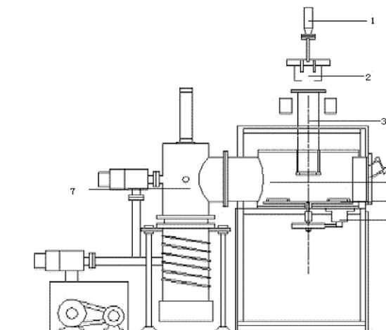
**Figure 1** - Schematic of the ion beam implantation device. 1. Air supply 2. Plasma generator 3. Ion beam 4. Big target chamber 5. Rotatable scaffold 6. Small target chamber 7. several vacuum pump
