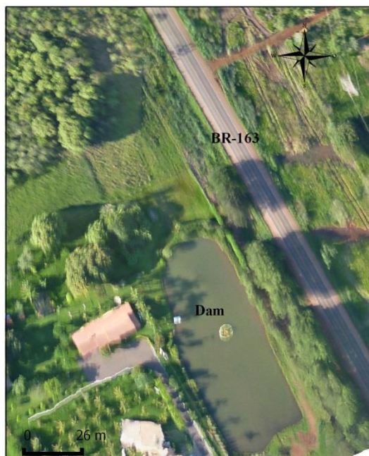
Figure 4: Orthorectified aerial photograph of water body #2, obtained by UAV. The image was used as reference for surface area and site identification. Acquisition date: November 17, 2012. Spatial resolution: 10 cm.
