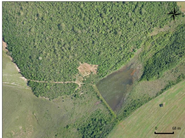
Figure 8: Orthorectified aerial photography of water body #3, obtained by UAV. The image was used as reference for surface area and site identification. Acquisition date: November 17, 2012. Spatial resolution: 16 cm.
