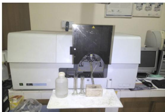
**Figure 3.** Atomic absorption spectrophotometer used for the analysis of heavy metals i.e zinc, lead, chromium and nickel present in the extracted tissues of muscles and gills.
