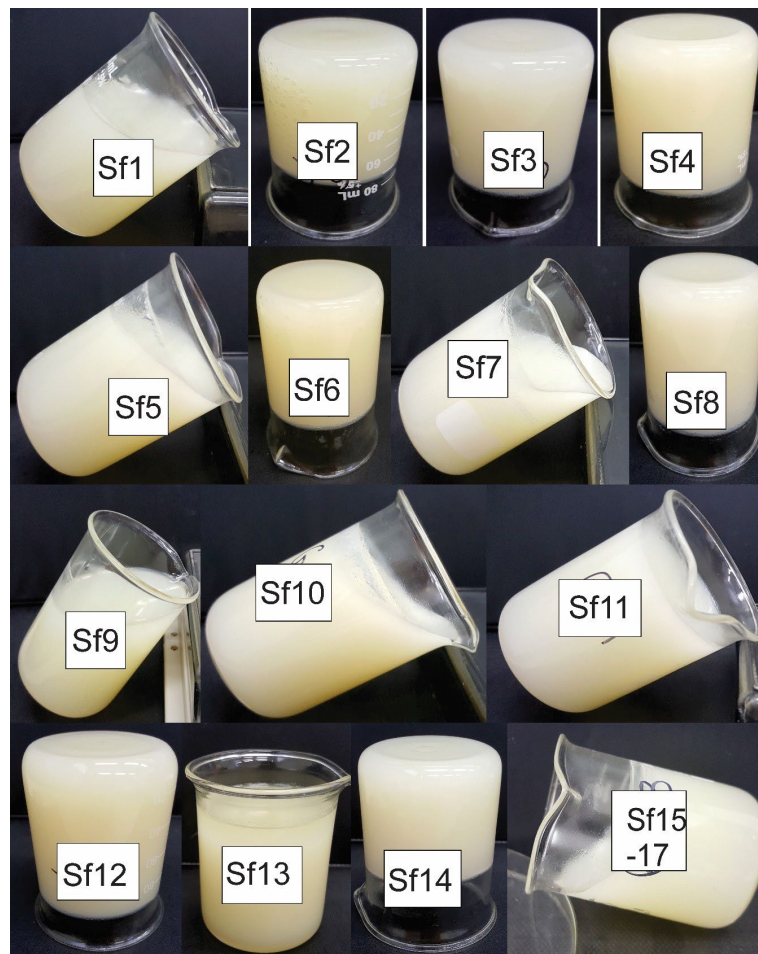
Figure 4. The visual appearance of the high sunflower oleogels (SF) at 25 °C after thermal stability, for samples concentration (1-17), please see Table 1.
