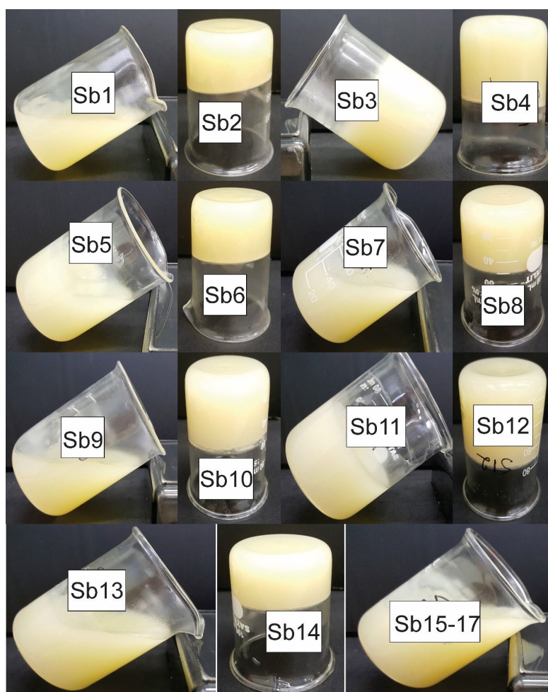
Figure 3. The soybean oleogels (Sb) visual appearance at 25 °C after thermal stability, for samples concentration (1-17), please see Table 1.
