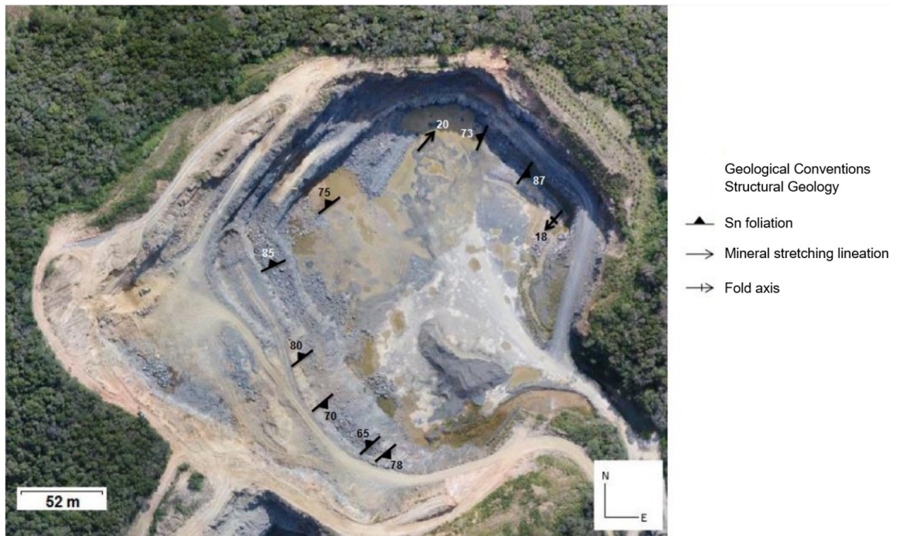
Figure 7. Main pit of the São Jorge quarry showing foliation and lineation measurements, modified from Saque (2017).
