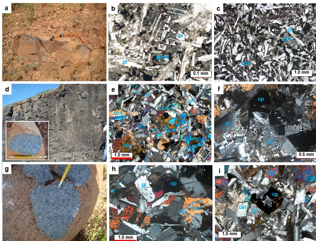
Figure 3. (a) Chilled margin of the Piripiri-Pedro II sill in contact with the Cabeças Formation sandstone (Stop GP-07), (b) interstitial glass to skeletal plagioclase crystals forming intersertal texture in the basalt of the Piripiri-Pedro II sill chilled margin (Stop GP-07), crossed nicols, (c) intergranular texture in the basalt from the border of the well 1-UN-26-PI (66.5 m deep), (d) diabase from the Batalha sill (approximate thickness at this point 40.0 m – Stop GP-24) exposed in quarry, (e) intergranular texture in diabase showing clinopyroxene in the interstices among tabular plagioclase, crossed nicols (Stop GP-24), (f) granophyric texture in diabase of the well 1-UN-26-PI (72.8 m deep), (g) gabbro from the Batalha sill (Stop GP-21), (h) subophitic texture in the gabbro of the well 1-UN-26 (96.2 m deep), (i) granophyric texture in the gabbro of the Batalha sill (Stop GP-25).
