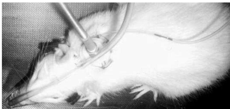
Figure 1. Rat connected to a metabolic mask and flow probe for oxygen consumption and cardiac output measurements.
