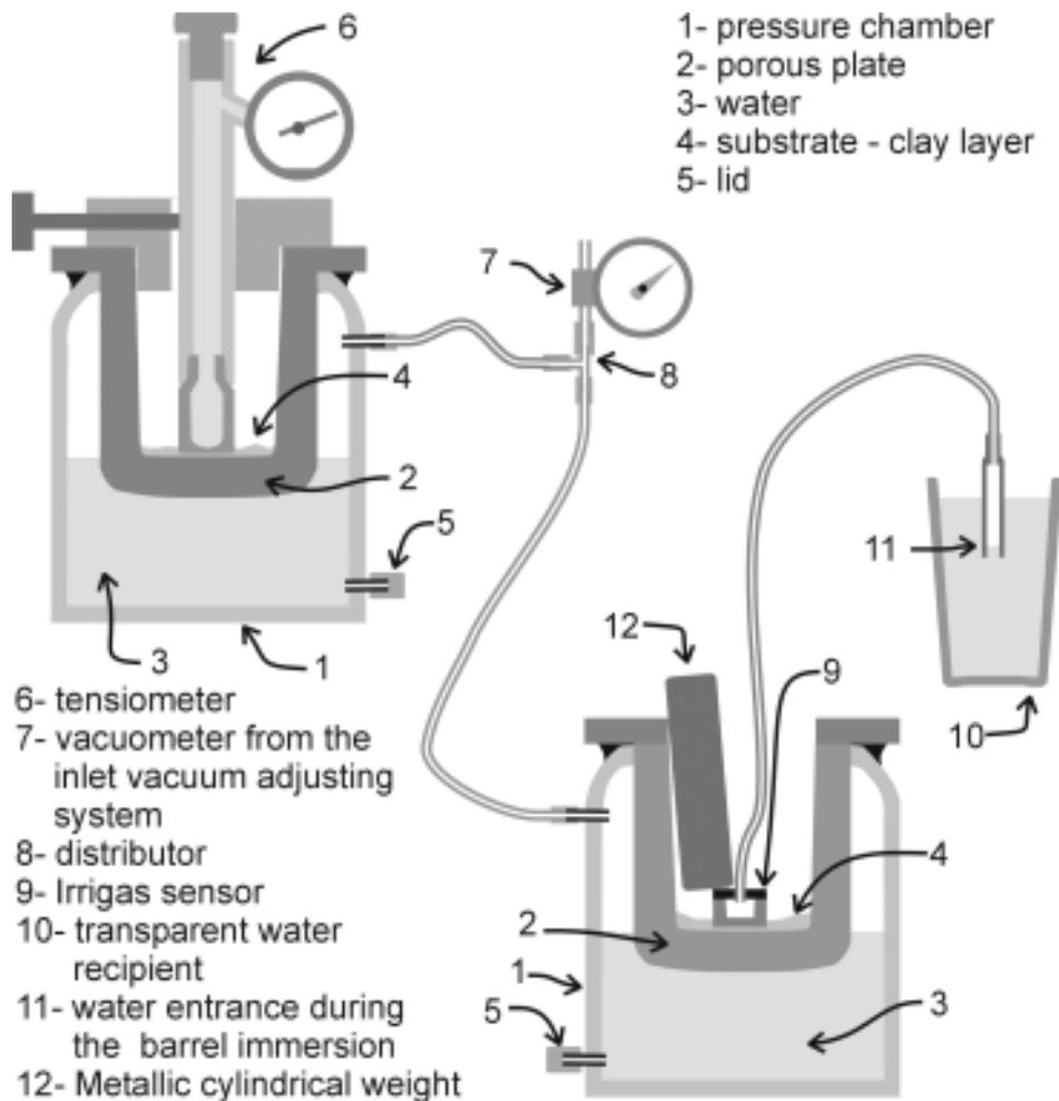
**Figure 2.** Illustration of two modified Richards negative pressure chambers, in which water tension of an irrigas sensor and of an conventional water filled-tensiometer are controlled simultaneously.
