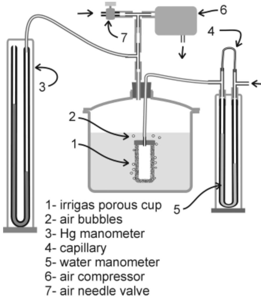
**Figure 3.** System with a capillary flowmeter to measure air-flow through an irrigas porous cup as a function of the applied gas tension. Arrows without numbers indicate the air flow direction in the system.
