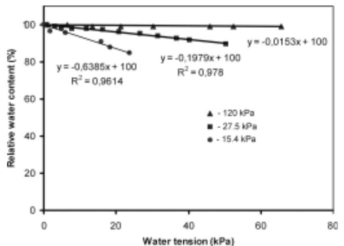
Figure 7. Relative water content of three porous cups as a function of water tension. The desorption critical water tension (Td) of the cups are ● -15.4 kPa, ■ - 27.5 kPa and ▲ - 120 kPa.
