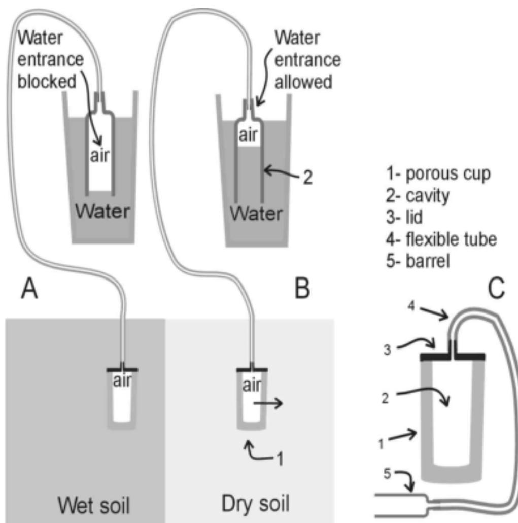
**Figure 1.** Illustration of the irrigas system to control irrigation. On the left side (A), in wet soil, the porous cup water imbibition does not allow the air permeation and water does not enter the barrel as it is immersed. In the center (B), in dry soil, there are opened paths for air permeation in the porous cup and, consequently, water enters the barrel during the immersion. On the right (C) an enlarged porous cup with details.
