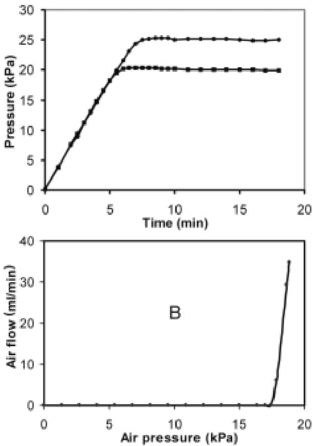
Figure 6. A- Typical trace for pressure as a function of time for a 25 kPa E-design irrigas porous cup immersed in water and subjected to an air-flow of 1.0 ml min<sup>-1</sup>. Circle (●) is for a irrigas porous at an water tension adjusted to zero and square (■) for the same irrigas porous cup at a water tension adjusted to 5 kPa. B- Typical trace for air-flow as a function of the applied air-pressure for a 17 kPa irrigas porous cup from the same maker immersed in water.
