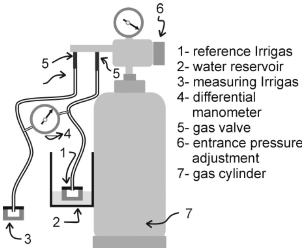
**Figure 4.** Differential steady gas flow driven irrigas tensiometer for direct soil water tension measurement.
