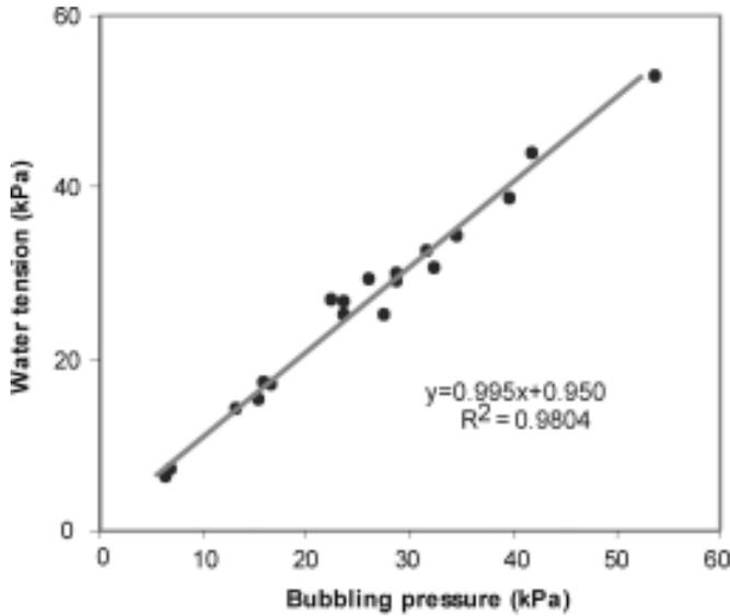
Figure 5. Soil water tension in which irrigas porous cups featuring different Td values (bubbling pressure) became air permeable.
