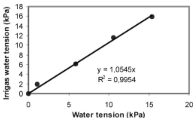
**Figure 8.** Typical response for a differential gas flow driven irrigas tensiometer to soil water tensions adjusted with a Richards pressure chamber.
