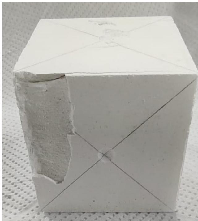
Figure 2: Image of a specimen with the GH4 treatment indicating the region from which the surface sample was extracted.
