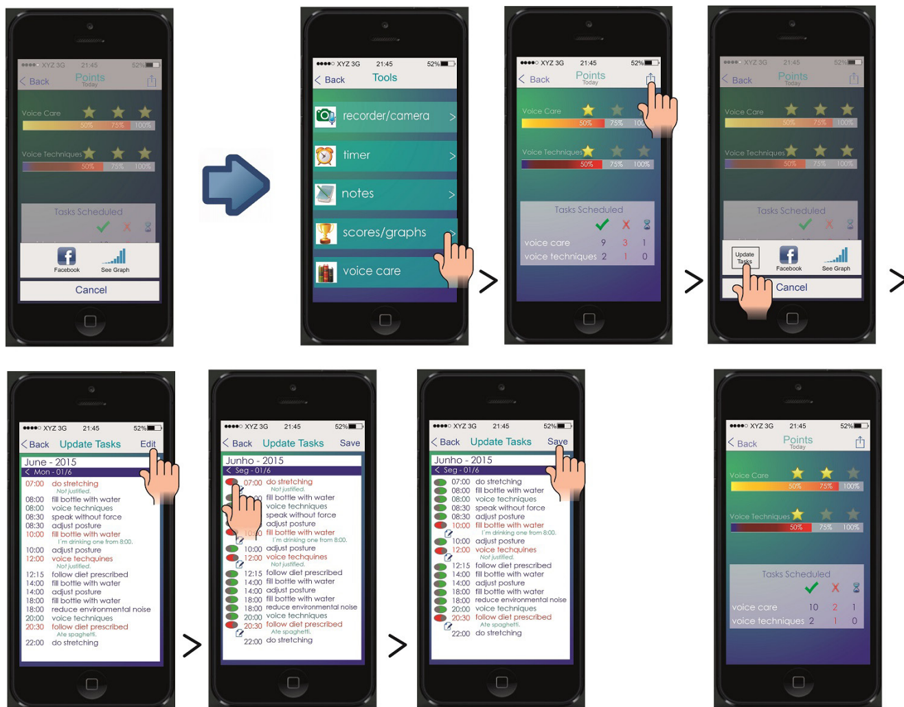
Figure 5. Modification to the prototype app: new screens for changing status of schedule activities. Source: Produced by authors
