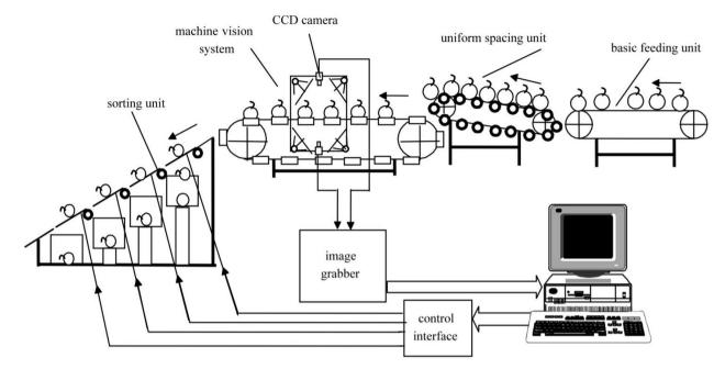
Figure 3. The application of computer vision in the representation of apple defects sorting system (Li et al., 2002).
