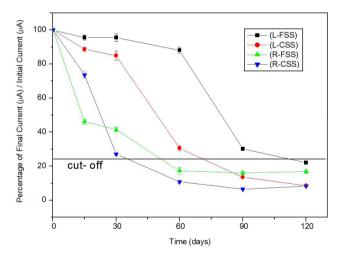
**Figure 2**. Percentage of decrease of the cathodic current of the devices after storage into a formulated (FSS) and commercial stabilizer solution (CSS) over time (15; 30; 60, 90 and 120 days) at refrigerated (4 °C) and room (25 °C) temperature.
