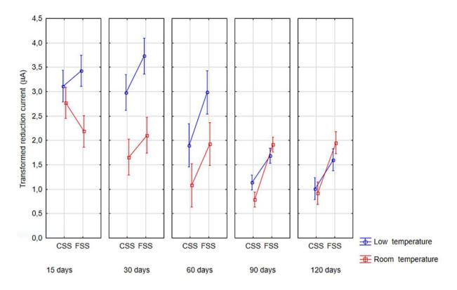
**Figure 1**. Confidence interval of the biosensor response in milk contaminated with *S*. Typhimurium (106 CFU.mL-1), transformed values, for interaction Time x Solution x Temperature after storage of the immunosensors in a commercial stabilizer solution (CSS) and a formulated stabilizer solution (FSS) in 15; 30; 60 and 90 and 120 days at room (25 °C) and low (4 °C) temperature. The standard deviation is shown for n = 10.
