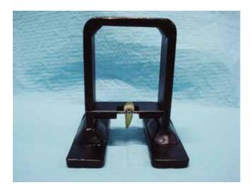
Figure 1 - Guide for standardization of test specimens (GSTS).
